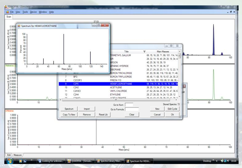
Continuously stored data may be interrogated at any time and correlated with known spectra either from the built in spectra library data base or from a remote spectra source such as NIST.
