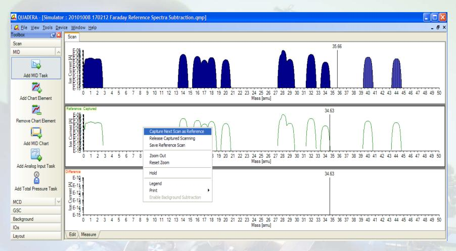
This mode enables the operator to monitor a process for any changes that may occur. Any difference in gas composition can easily be logged and displayed on the bottom "Difference" axis. The acquired spectra may be interrogated and compared with a spectra library for identification of new, evolved gas species at any time.
