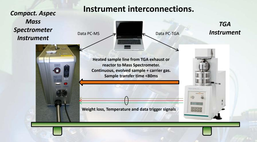
The Aspec, bench top, Mass Spectrometer is connected directly to the TGA instrument via a 3m signal cable and heated sample line as shown above.
