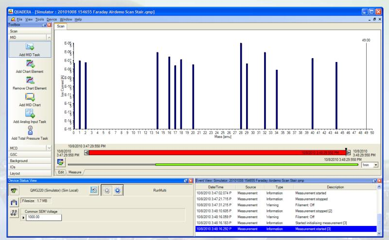
In this mode, you can "scan" the entire mass range of the instrument in less than 2 seconds and produce a complete spectra of any gas composition. The spectra will automatically show very low as well as very high concentrations all on one single spectra. Each bar of the graph above represents a different gas or isotope of a gas. The higher the signal, the more gas there is. This mode enables the user to quickly see if the gas composition is accurate and correct.
