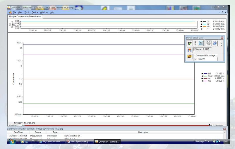
This mode the is the most commonly used mode. It enables the user to calibrate and display up to 64 gas species and measure in direct concentration. Each gas component is calibrated by a set up routine and once calibrated the instrument will measure, data log and display the data in real time.
