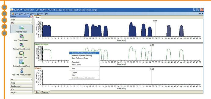
This screen shows a fast mass scan of all gases entering the instrument from a process. Note the aspec 1560 can measure across 9 decades of concentration ranges in a single scan. The instrument is therefore capable of measuring from ppb to 100% of many gas components with no modification. A full 200amu mass scan can be carried out in less than 4 seconds.
