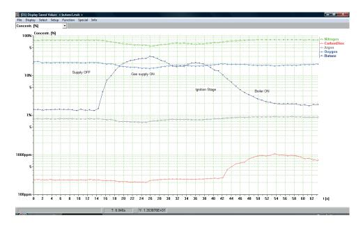
Absolute Concentration verses time values (ppb, ppm, %) are possible by creating a matrix in software that contains the gas component, the relevant mass number/s and the maximum span concentration of the gas component of interest. There is only a need for a single "span" gas mixture to be provided to make a calibration of concentration and takes only a few seconds to perform. It is also possible to make a "zero" gas calibration if extra low concentration are expected within the analysis.
