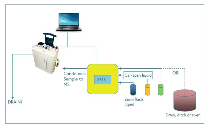
The RMS unit is a robust, self contained liquid sampler consisting of several electronic sample valves, Variable sample rate Peristaltic Pump. Logic control and sample stream indicators.
