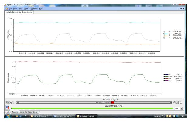
Note again the ability of the fast sample system as well as the ability of the MS to plot data points at 2ms intervals! The profile of <u>each breath</u> can now be seen again!
