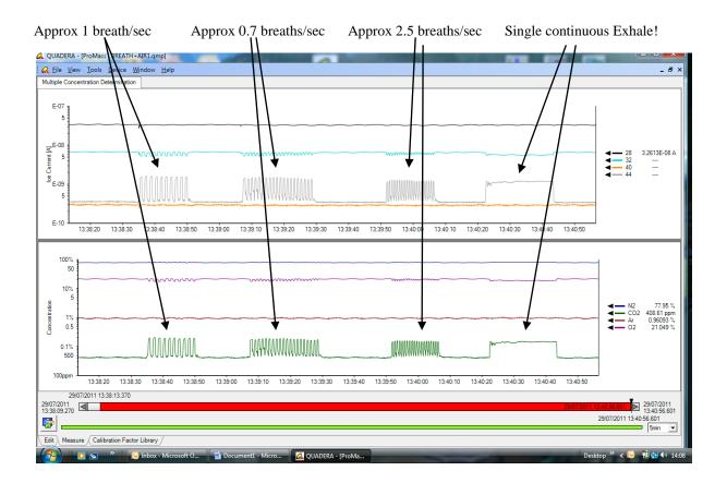
As can be seen, both the inlet gas transfer speed and also the ability of the MS to plot data points at 2ms intervals enable you to clearly analyse the shape and profile of <u>each individual breath!</u>
