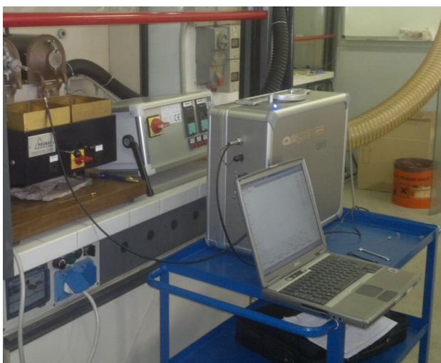
Figure 1. Aspec Ltd MIMS system installed in the University of Milan. Measuring gas produced by the roasting process of coffee beans.
