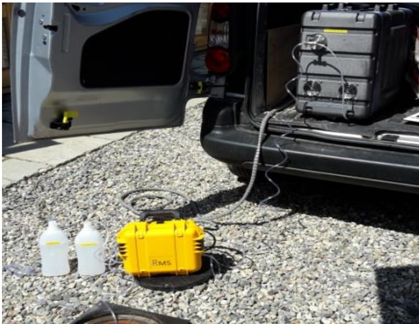
Figure 5. Aspec ltd MIMS instrument with RMS attachment (yellow instrument) deployed in bore hole. A 1 litre bottle of flush (water and detergent) and a 1 litre bottle of calibration fluid. (distilled water).
